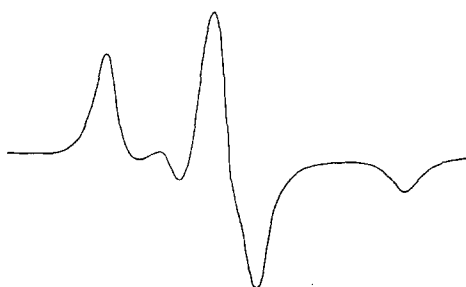
Fig. 2(b). Spectrum of the BHT-amino TEMPO in a rigid medium (solution deep-frozen at 180 K in liquid nitrogen).
